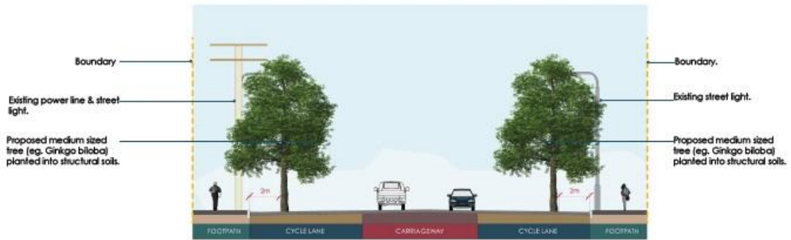
SUB-ARTERIAL LOCATION TYPE 4 | SECTION
