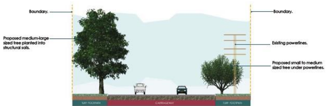
COLLECTOR ROAD LOCATION TYPE 6 | SECTION
