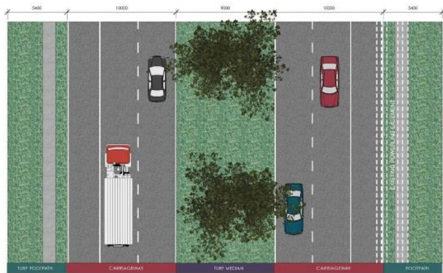
SUB-ARTERIAL LOCATION TYPE 5 | DETAIL PLAN
